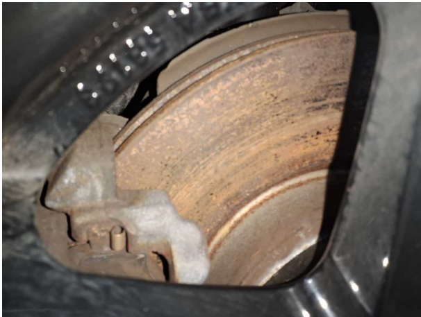
Damage #6: Braking system: Brake discs and brake pads - front - Corrosion - Replace
