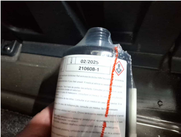
Damage #1: Equipment: Tirefit filler - Expired - Replace
