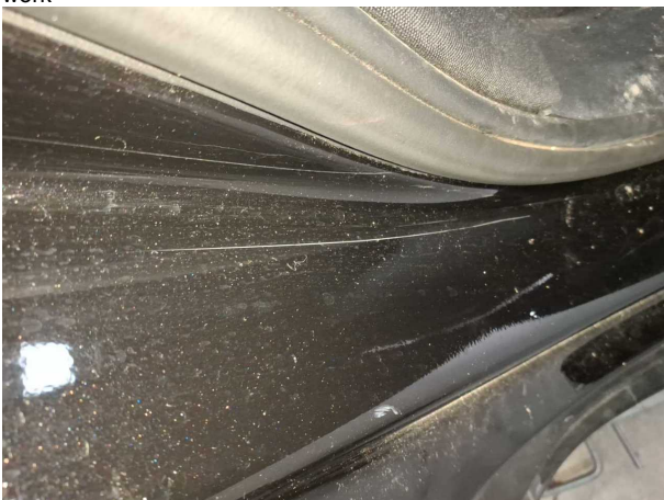
Damage #3: Side panel - rear right side: Sill - Scratch(es) - Smart repair
