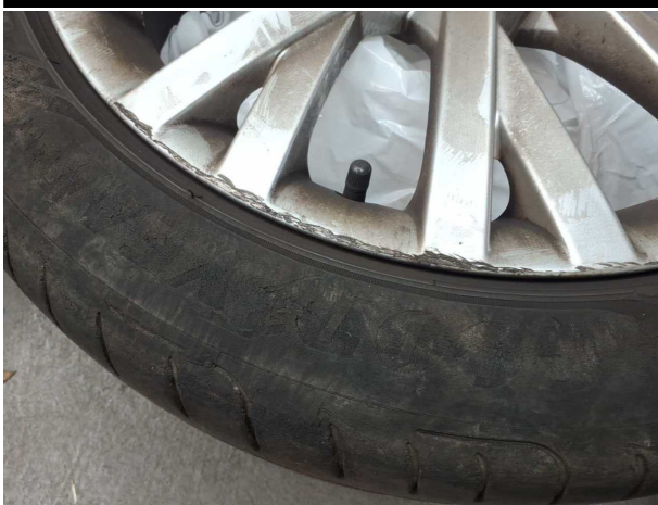
Damage #4: 2nd wheel set: 1 alloy rim - Damaged - Loss in value
