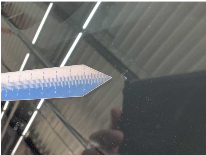
Wear and tear 3: Vehicle glazing: Windscreen with lane departure assistant - Stone chips - No deduction
