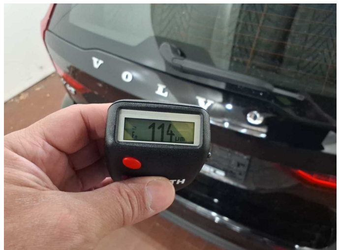
Repainting 1: Boot lid / rear door
