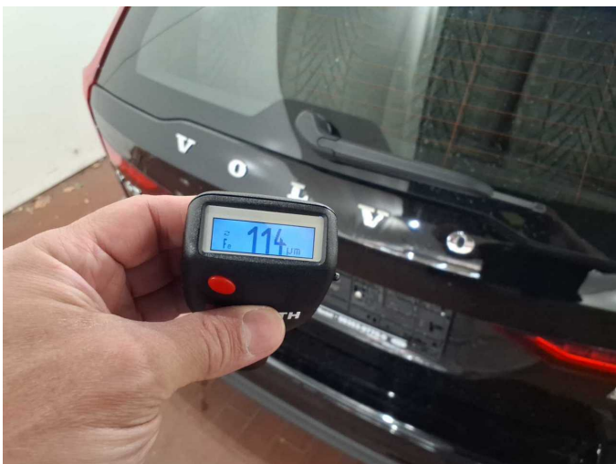
Repainting 1: Boot lid / rear door
