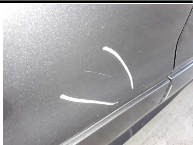
Damage #13: Sliding door, right: Sliding door with glass panel - Scratched - Repair and paint
