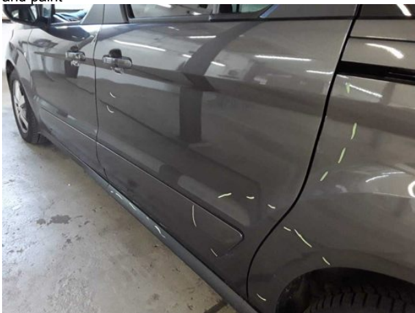
Damage #12: Sliding door - left side: Sliding door with glass pane... Scratched - Repair and paint
