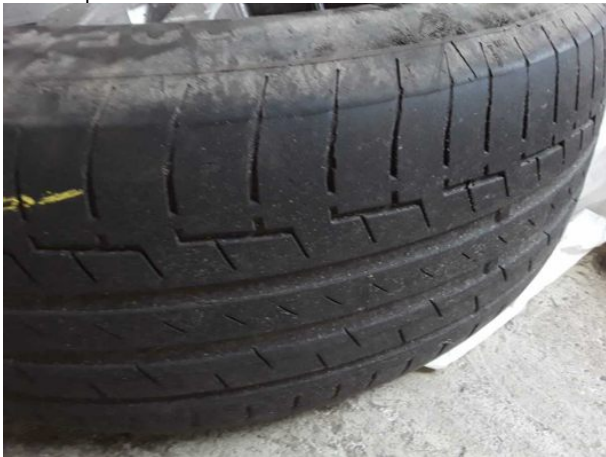
Damage #8: 2nd wheel set: 2 tyres - Worn - Replace
