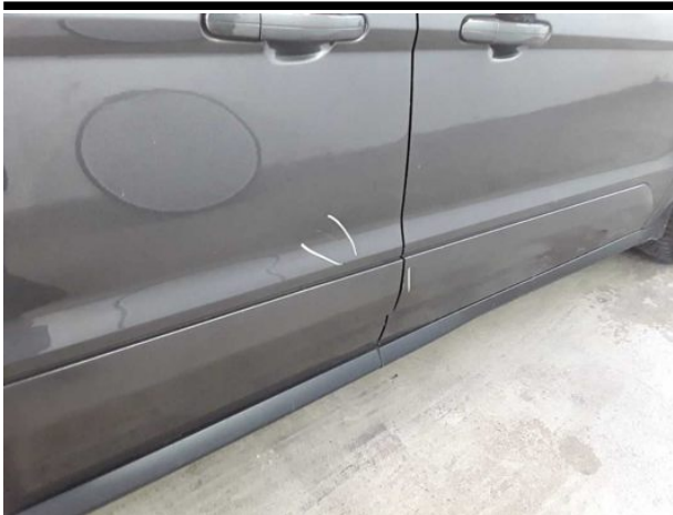
Damage #13: Sliding door, right: Sliding door with glass panel - Scratched - Repair and paint
