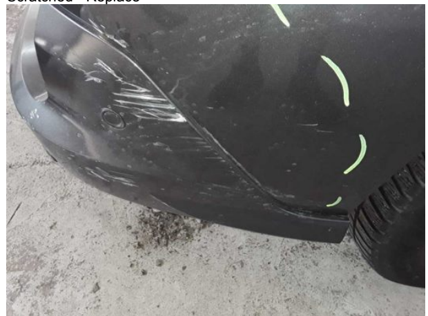
Damage #15: Rear bumper: Rear bumper (Verformt) - Scratched - Replace
