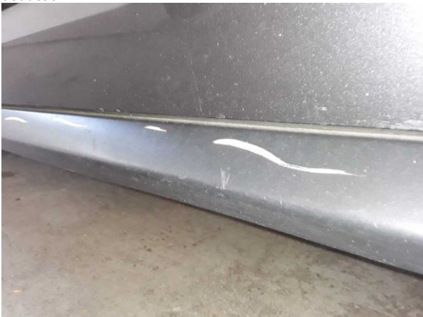
Damage #3: Sill - left side: Trim - Scratched - Loss in value
