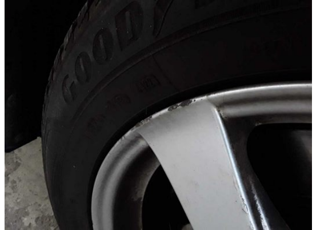
Damage #1: Wheel / tyres: Alloy rim - front right side - Scratched - No deduction
