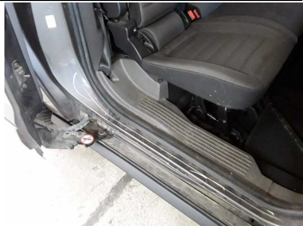
Damage #11: Side panel - rear right side: Sill - Scratched - Repair and paint
