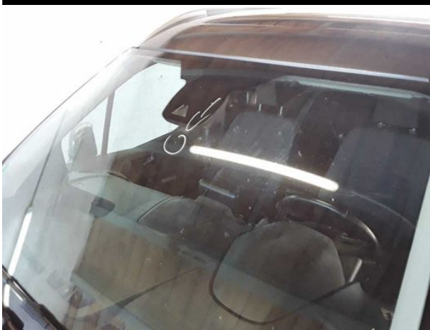
Damage #16: Vehicle glazing: Windscreen, heated (Rissbildung) - Stone chips - Replace
