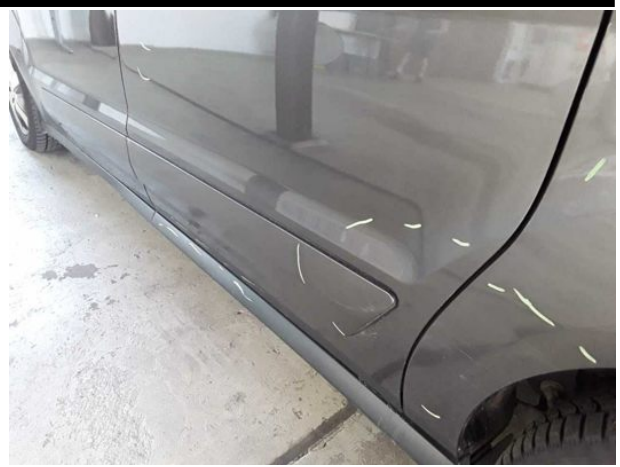
Damage #5: Door - rear left side: Brightware - lower - Scratched - Smart repair
