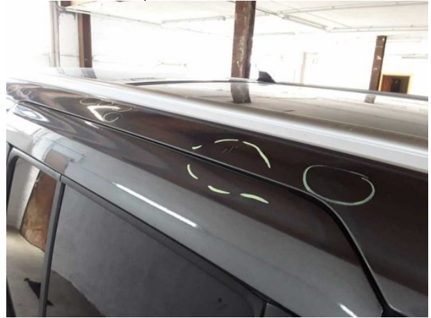
Damage #6: Roof: Roof rail - right side - Scratched - Smart repair
