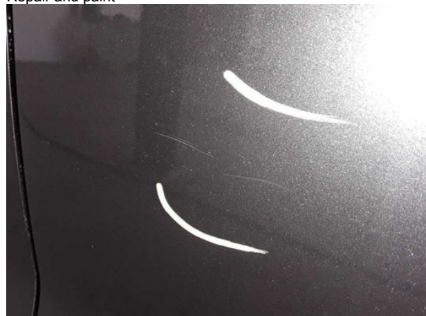
Damage #12: Sliding door - left side: Sliding door with glass panel - Scratched - Repair and paint
