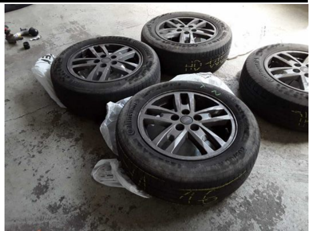
Damage #8: 2nd wheel set: 2 tyres - Worn - Replace
