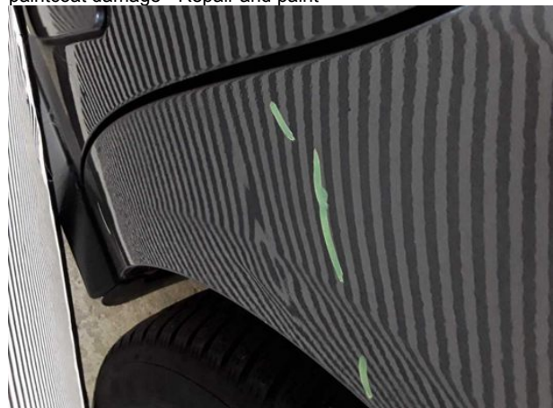
Damage #14: Side panel - rear left side: Side panel - Dent / paintcoat damage - Repair and paint
