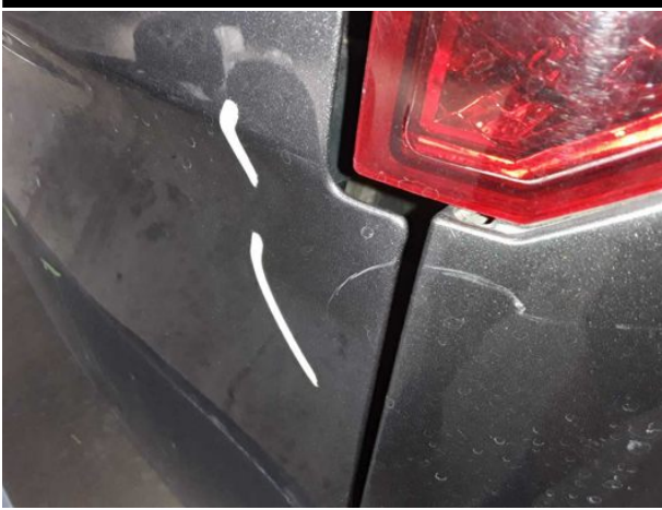
Damage #4: Boot lid / rear door: Boot lid - Scratched - Smart repair
