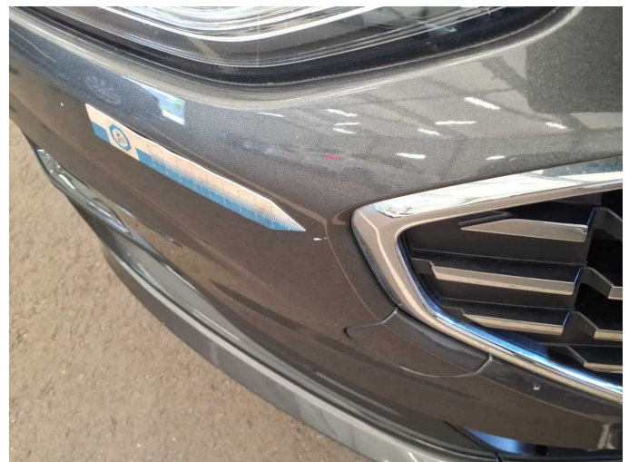
Damage 3: Front bumper: Front bumper - Scratch(es) - Paint
