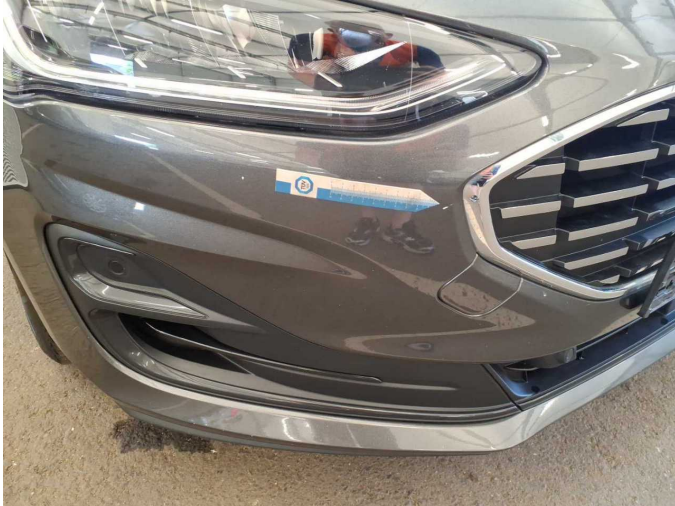
Damage 3: Front bumper: Front bumper - Scratch(es) - Paint
