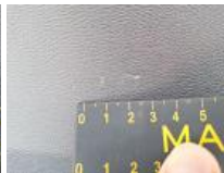
Boot lid covering R, Scratch(es), Replace
