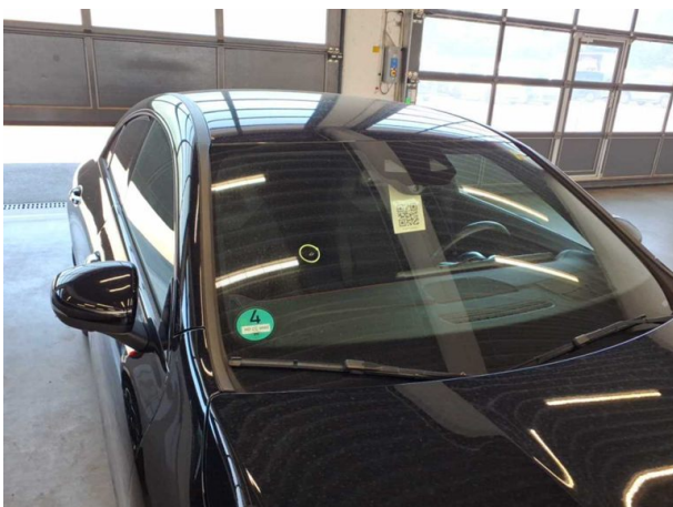
Damage #9: Vehicle glazing: Windscreen with lane departure assistant (Mit rissbildung) - Stone chips - Replace
