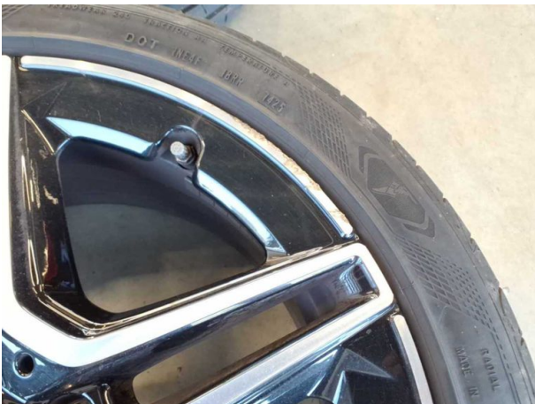
Damage #3: 2nd wheel set: 1 alloy rim (Materialabtrag optisch zu hoch) - Scratched - Loss in value
