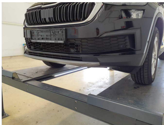
Damage 5: Front bumper: Spoiler - Broken / torn - Replace
