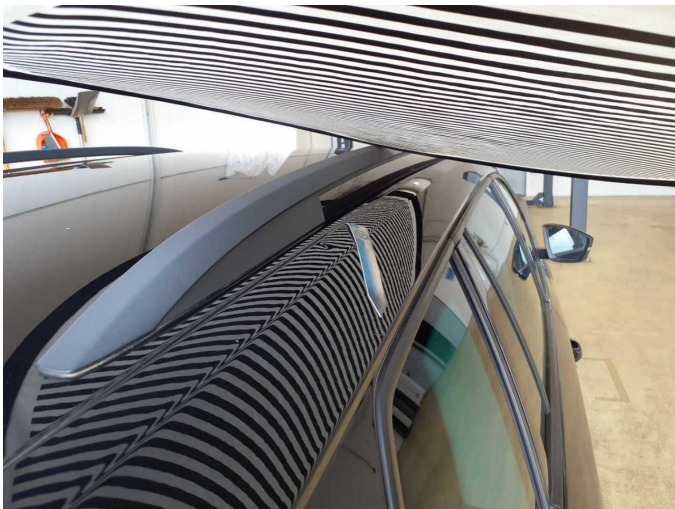
Damage 6: Roof: Roof rail - right side - Dent / paintcoat damage - Repair and paint
