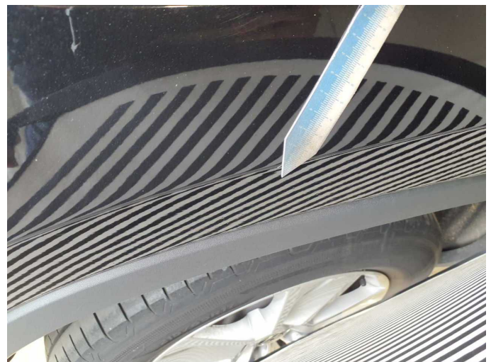
Damage 7: Side panel - rear right side: Side panel (Einschlüsse) - Unprofessionally repaired - Repair and paint
