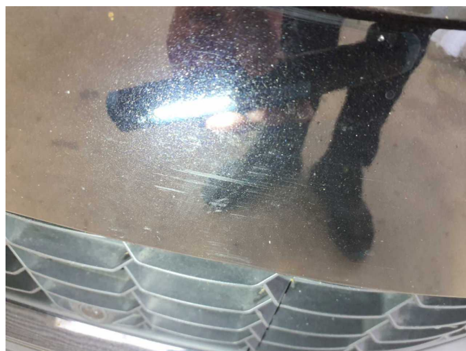
Damage 11: Front bumper: Front bumper - Scratch(es) - Paint
