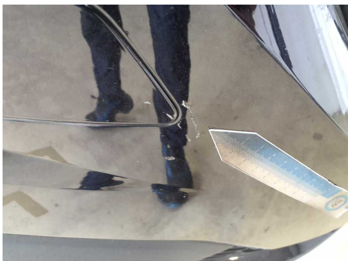
Damage 11: Front bumper: Front bumper - Scratch(es) - Paint
