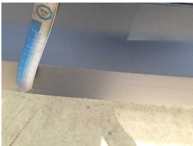
Damage 4: Rear bumper: Spoiler - Scratch(es) - Replace
