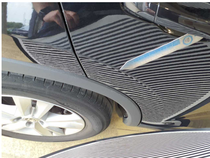
Damage 10: Door - rear right side: Door (Wellig) - Unprofessionally repaired - Repair and paint
