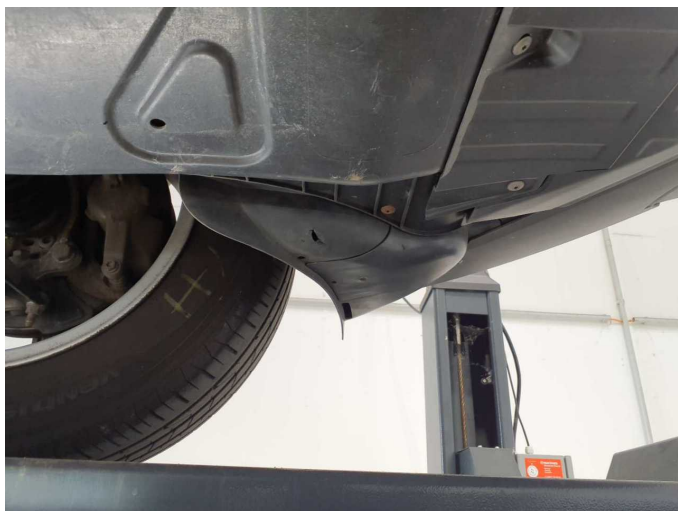
Damage 3: Body: Wheel well - front left side - Broken / torn - Replace
