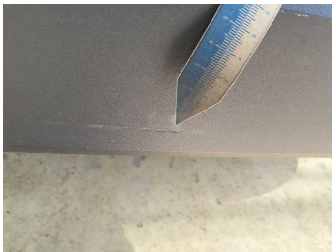
Damage 4: Rear bumper: Spoiler - Scratch(es) - Replace
