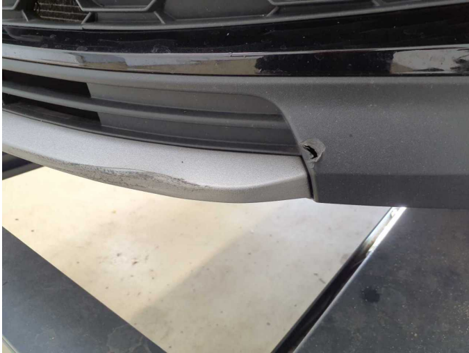
Damage 5: Front bumper: Spoiler - Broken / torn - Replace
