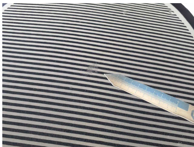
Damage 12: Bonnet: Bonnet (Anätzung) - Paint defect - Repair and paint
