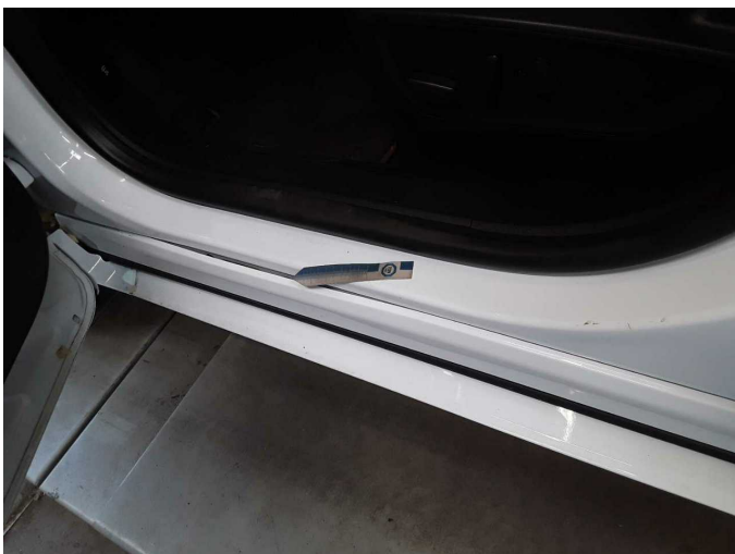
Damage 6: Sill - left side: Trim - Damaged - Replace
