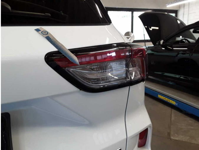
Damage 5: Tail light: Tail lamp - right side - Porous / cracked - Replace
