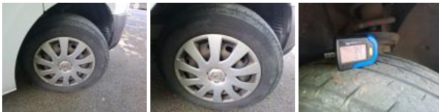
Tyre FL, Out of tolerance, Replace
