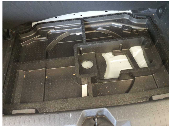
Missing part 2: Equipment: Tirefit complete - Missing - Replace
