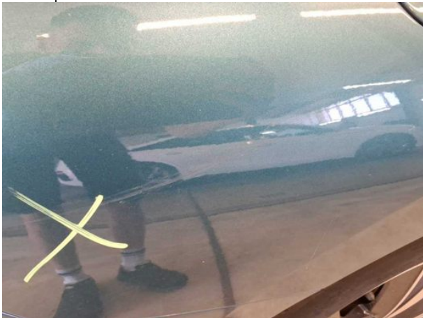
Damage #1: Side panel - rear right side: Side panel - Scratched - Cover / polish
