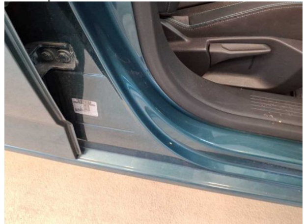
Damage #2: Sill - right side: Sill - dent(s) - Smooth repair work
