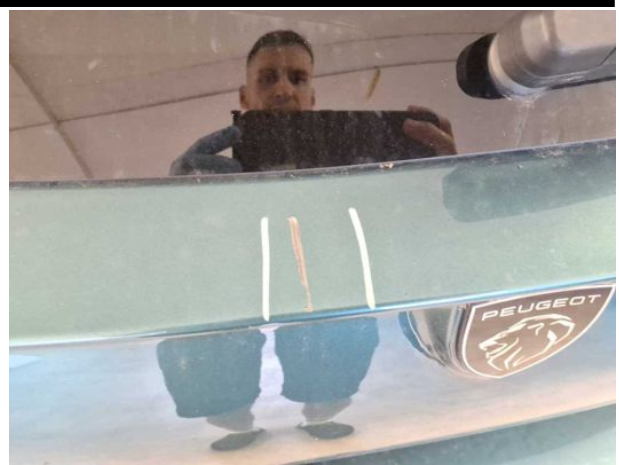
Damage #12: Boot lid / rear door: Boot lid - Scratched - Repair and paint
