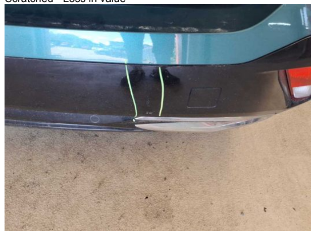
Damage #7: Rear bumper: Spoiler - Scratched - Replace
