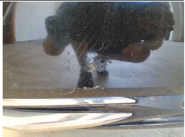
Damage #7: Rear bumper: Spoiler - Scratched - Replace
