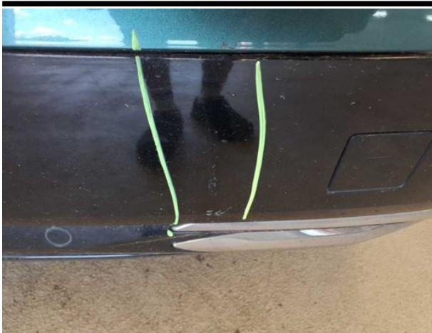
Damage #7: Rear bumper: Spoiler - Scratched - Replace
