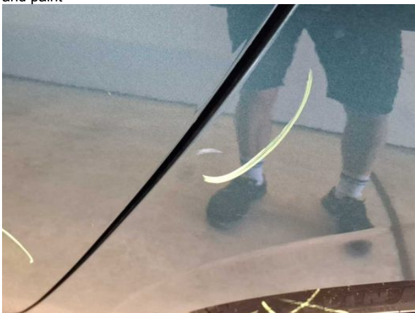
Damage #11: Side panel - rear left side: Side panel - Scratched - Repair and paint
