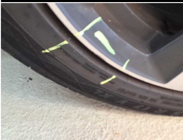
Damage #3: Wheel / tyres: Alloy rim - front left side - Scratched - Loss in value
