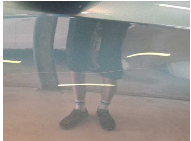
Damage #14: Door - front right side: Door - Scratched - Repair and paint
