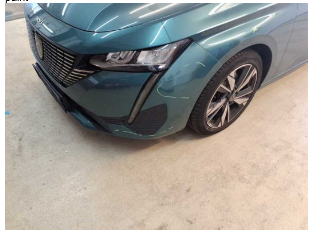
Damage #10: Front bumper: Front bumper - Scratched - Rep... and paint
