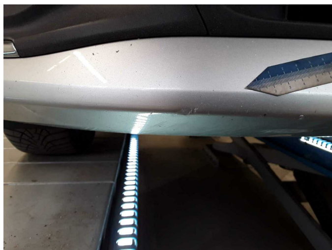
Damage 5: Front bumper: Front bumper - Scratched - Paint
