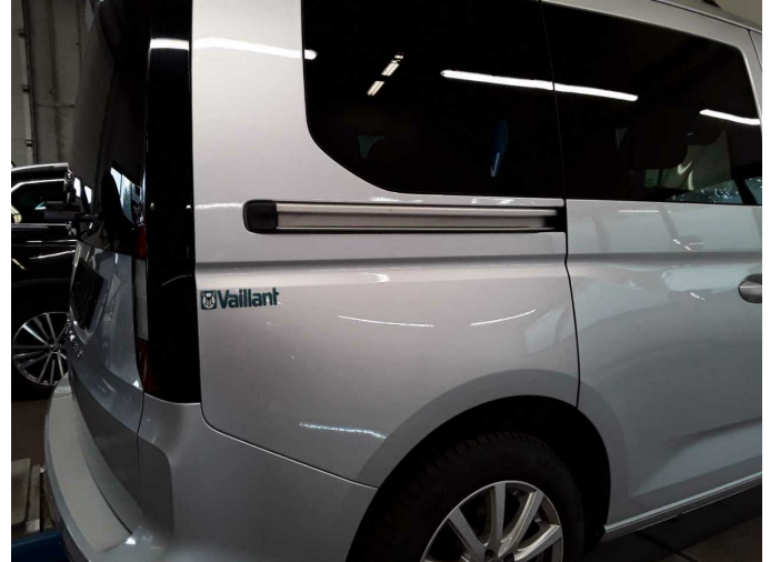
Damage 2: Side panel - rear right side: Side panel - Glued / labelled - De-glue / neutralise
