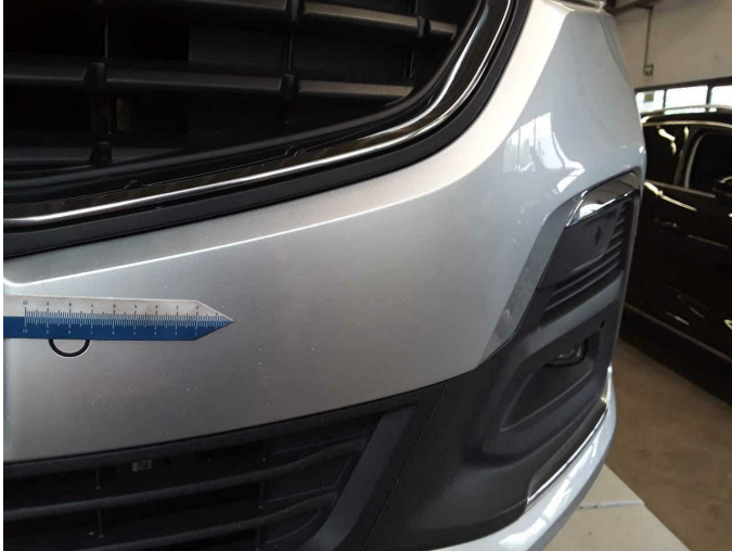
Damage 5: Front bumper: Front bumper - Scratched - Paint
