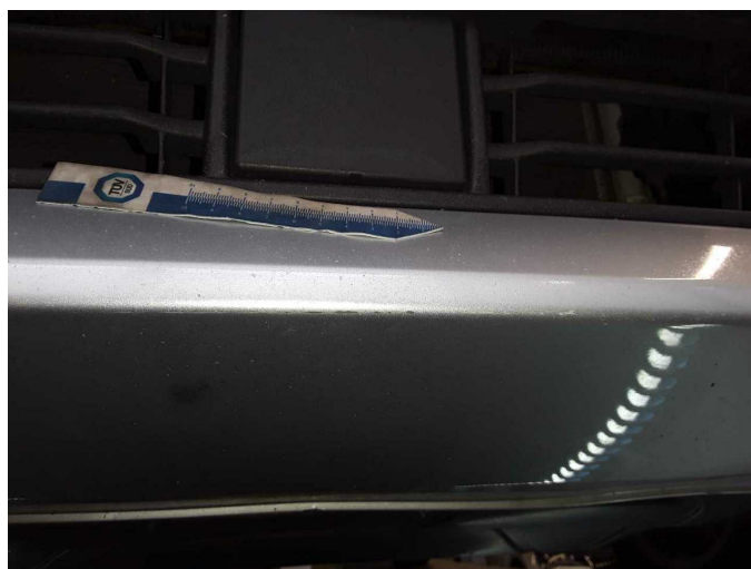
Damage 5: Front bumper: Front bumper - Scratched - Paint
