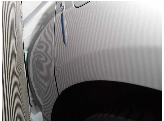
Damage 6: Side panel - rear left side: Side panel (Schleifspuren, wellig) - Unprofessionally repaired - Repair and paint
