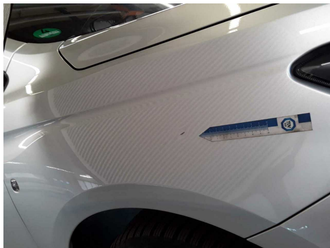
Damage 4: Mudguard - right side: Mudguard - right side - Dent / paintcoat damage - Smart repair
