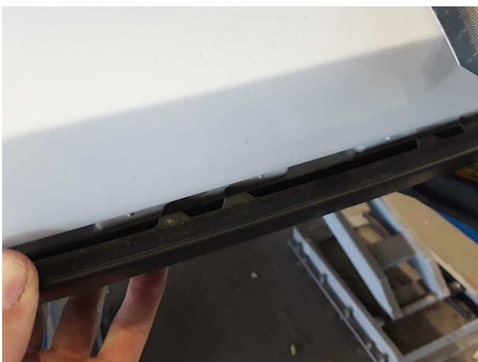
Damage 3: Rear bumper: Spoiler - Damaged - Replace
