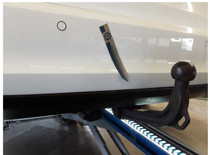
Damage 3: Rear bumper: Spoiler - Damaged - Replace
