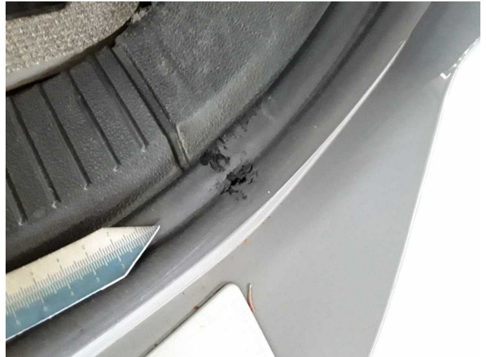
Damage 3: Cab: Door rubber seal - left side (Heckklappe) - Damaged - Replace
