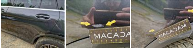
Door FL, Dent(s), Repair and paint (complete)
