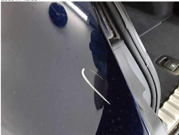
Damage #10: Side panel - rear left side: Side panel - Scratched - Smart repair
