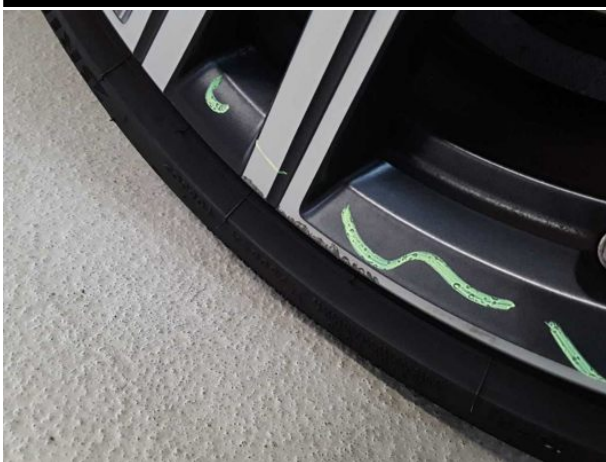
Damage #9: Wheel / tyres: Alloy rim - front right side - Scratched - Loss in value
