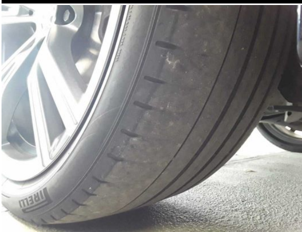
Damage #12: Wheel / tyres: Tyre - right - Worn - Replace
