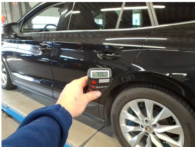
Repainting 7: Door - rear left side
