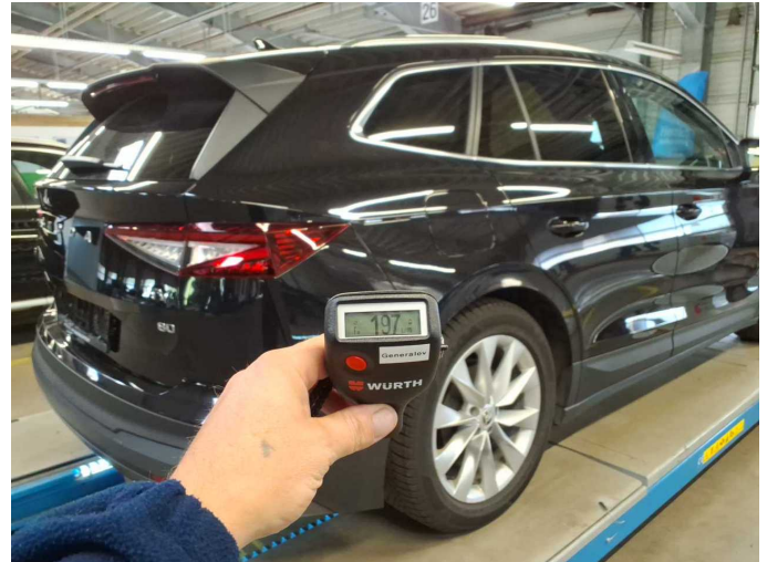
Repainting 6: Side panel - rear right side
