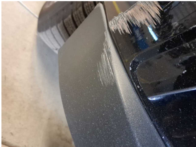
Damage 13: Front bumper: Spoiler - Scratched - Replace
