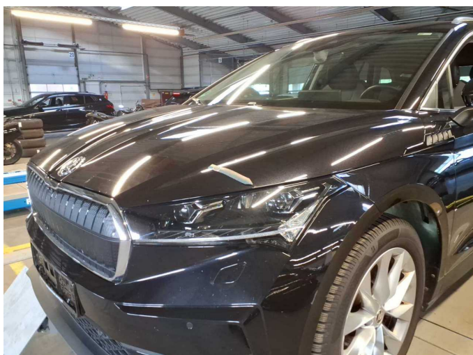
Damage 16: Bonnet: Bonnet (Rostbildung) - Stone chips - Repair and paint
