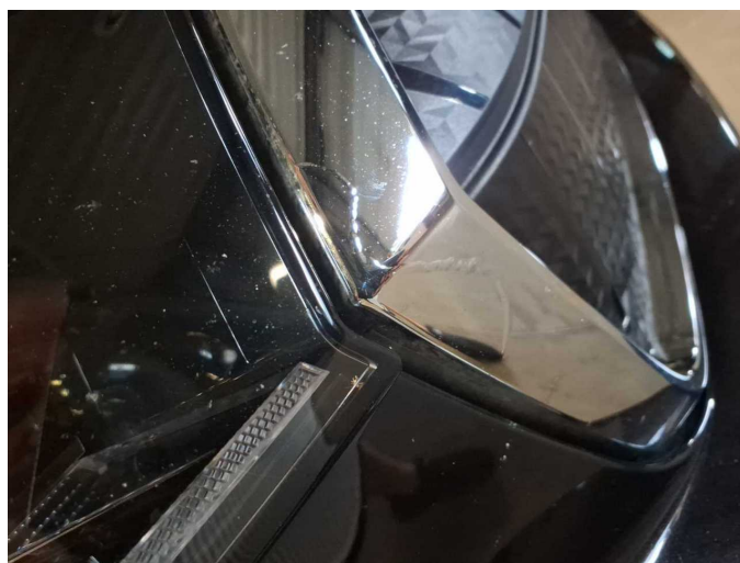
Damage 14: Bonnet: Radiator grille (Rahmen) - Paint defect - Replace
