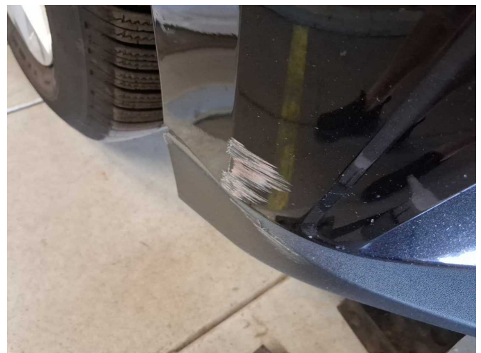
Damage 13: Front bumper: Spoiler - Scratched - Replace
