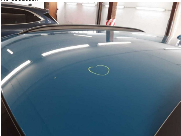
Damage #3: Roof: Roof - dent(s) - Smooth repair work
