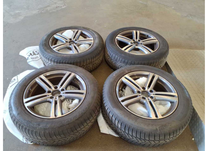
Missing part 2: 2nd wheel set: Wheel cover set - complete (Nabendeckel) - Missing - Replace
