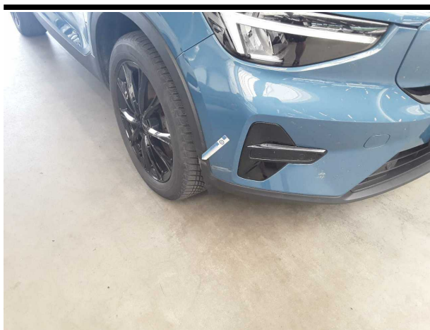
Damage #5: Front bumper: Spoiler - Deformed - Replace
