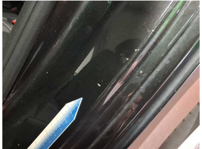
Damage 5: Side panel - rear left side: Sill - Dent / paintcoat damage - Smart repair
