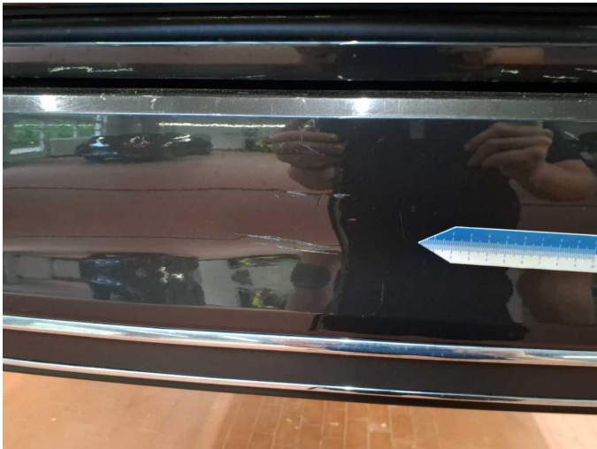
Damage 12: Rear bumper: Rear bumper - Dent / paintcoat damage - Replace
