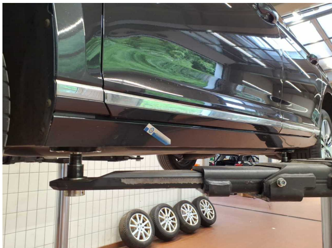
Damage 2: Sill - left side: Trim - Scratched - Smart repair
