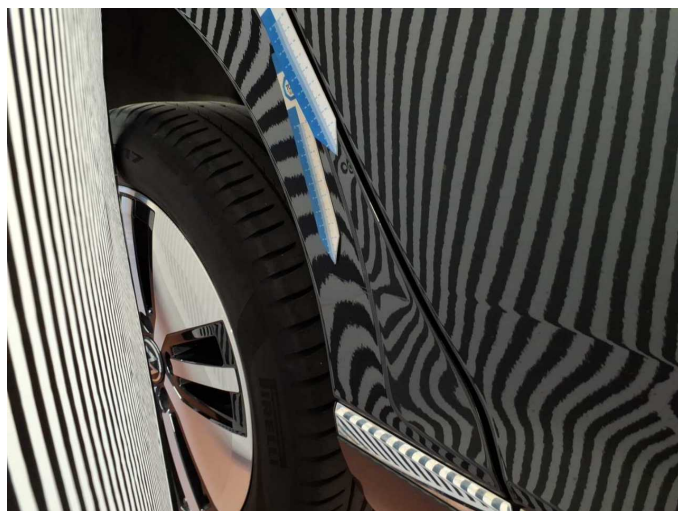
Damage 8: Side panel - rear right side: Elbow - Dent / paintcoat damage - Repair and paint
