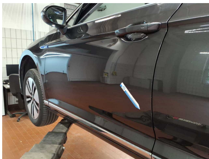
Damage 4: Door - front left side: Door - dent(s) - Smooth repair work
