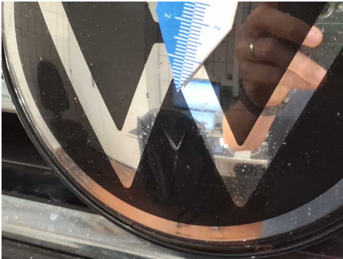
Damage 6: Front structure: Emblem - Broken / torn - Replace
