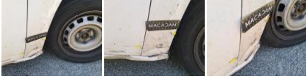
Outer sill R, Dent(s) and scratch(es), Replace and paint
