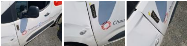
Outer sill L, Dent(s) and scratch(es), Repair and paint (complete)
