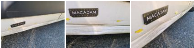
Bumper corner RL, Broken, Replace
