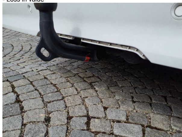
Damage 6: Rear bumper: Cover - bumper - rear - Missing - Replace
