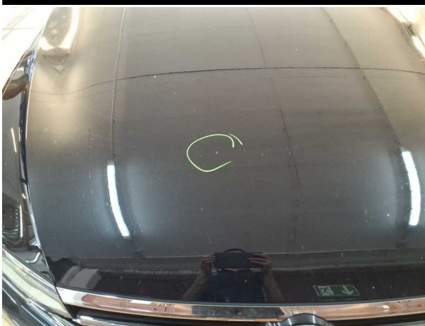
Damage #5: Bonnet: Bonnet - Dent / paintcoat damage - Repair and paint
