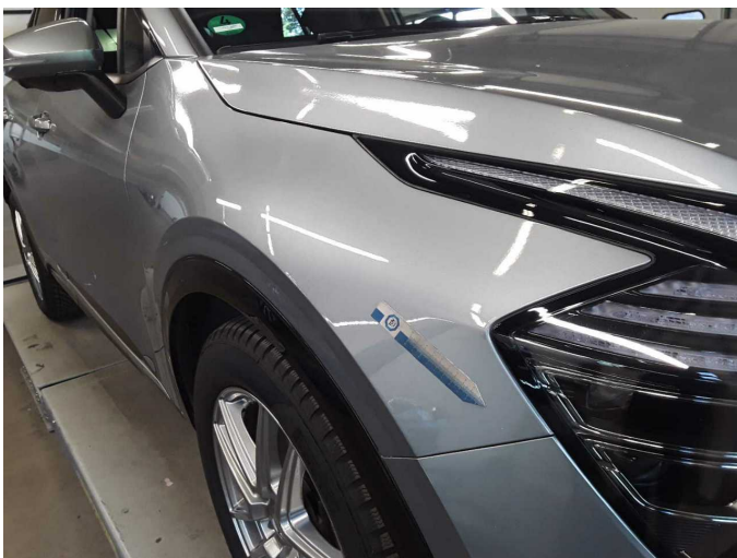
Wear and tear 2: Mudguard - right side: Mudguard - right side - Stone chips - No deduction
