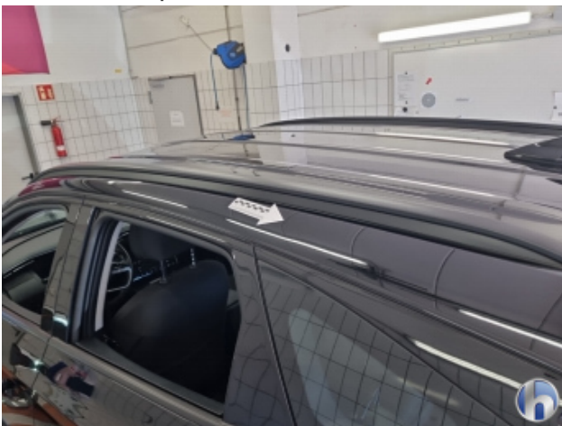
2. Dachrahmen - Links 1 Delle - Sanft Instandsetzen
