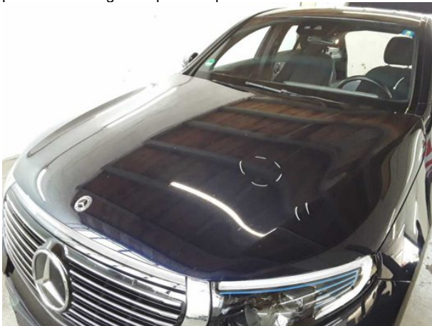
Damage #17: Bonnet: Bonnet - Scratched - Repair and paint
