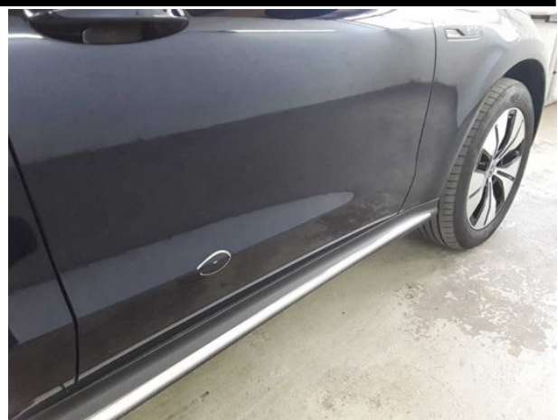
Damage #11: Door - front right side: Door - Scratched - Smart repair
