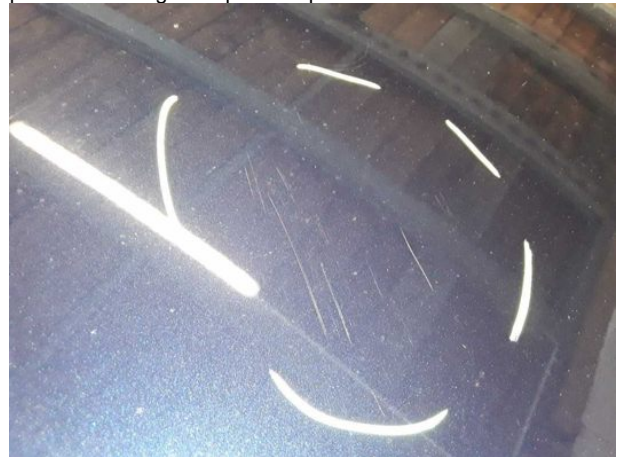
Damage #17: Bonnet: Bonnet - Scratched - Repair and paint
