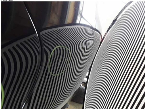
Damage #12: Side panel - rear left side: Side panel - dent(s) - Smooth repair work
