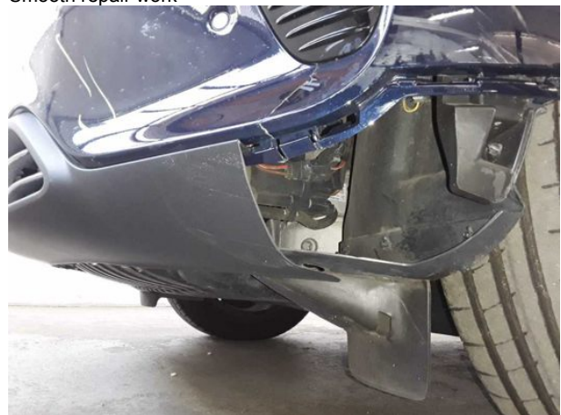
Damage #13: Front bumper: Spoiler - Damaged - Replace
