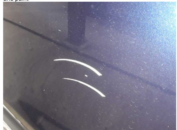
Damage #15: Door - front left side: Door - Scratched - Repair and paint
