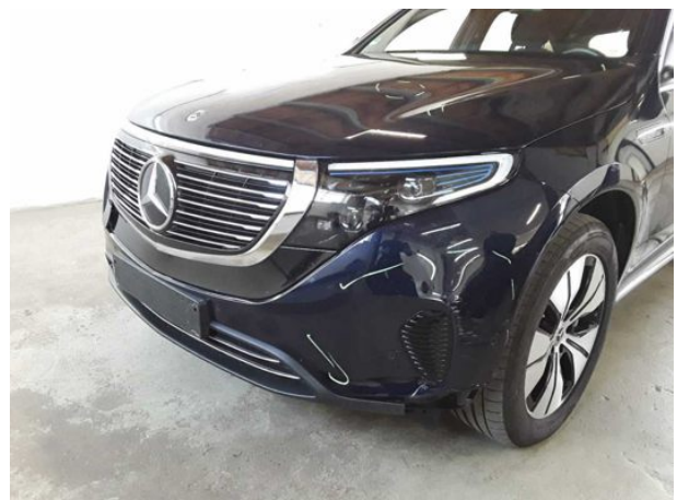
Damage #18: Front bumper: Bumper with Parktronic - Damaged - Replace
