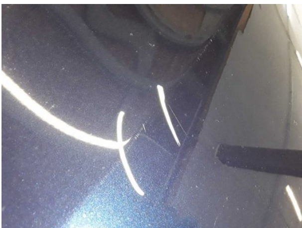
Damage #17: Bonnet: Bonnet - Scratched - Repair and paint
