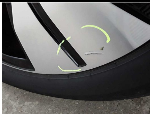
Damage #8: Wheel / tyres: Alloy rim - rear right side - Scratched - Loss in value
