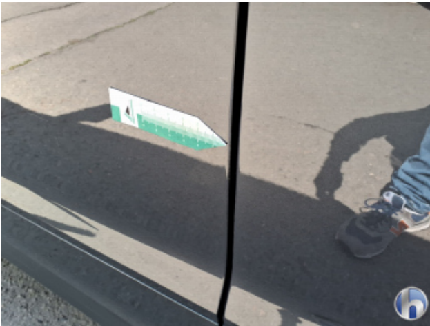
2. Tür Vorne - Links Kratzer - Smart Repair
