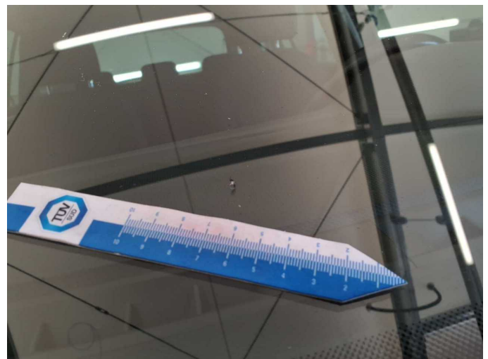
Damage 5: Vehicle glazing: Windscreen - Stone chips - Smart repair
