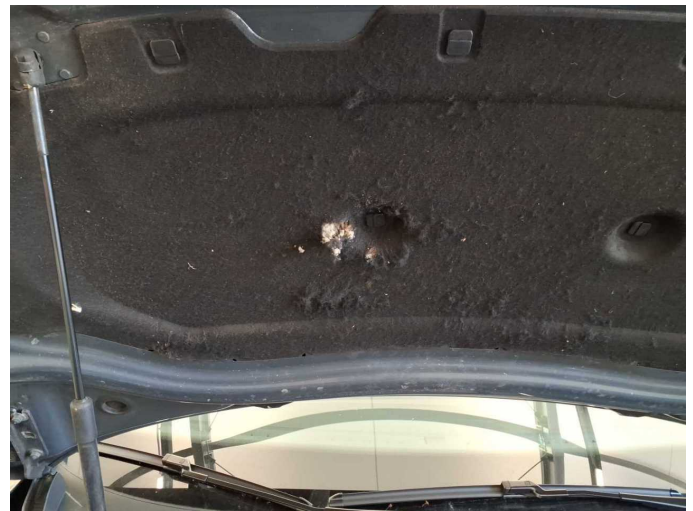
Damage 4: Bonnet: Insulation lining - Damage caused by marten / rodent - Replace
