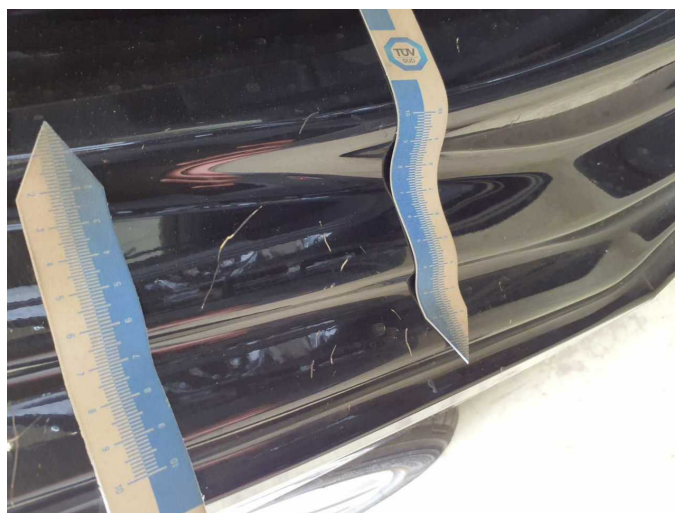
Damage 9: Side panel - rear right side: Sill - Scratch(es) - Paint
