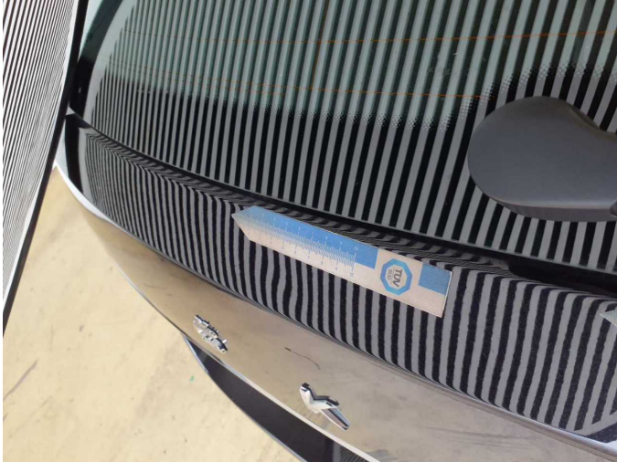
Wear and tear 7: Boot lid / rear door: Boot lid - dent(s) - Smooth repair work
