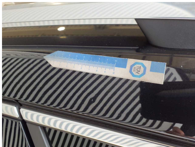
Damage 3: Roof: Roof rail - left side - Dent / paintcoat damage - Smart repair
