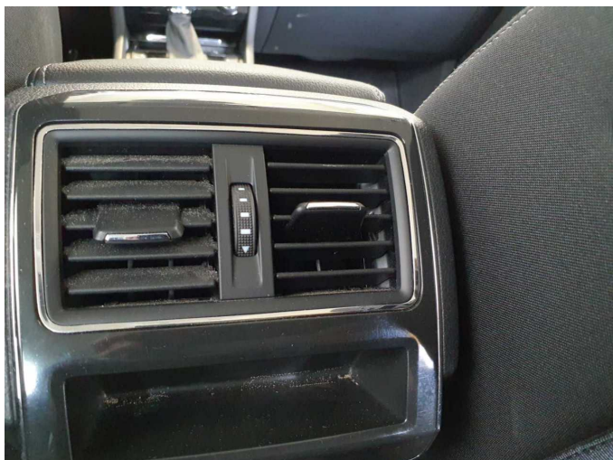
Damage 8: Instrument panel: Air nozzle - centre (Hinten) - Broken / torn - Replace
