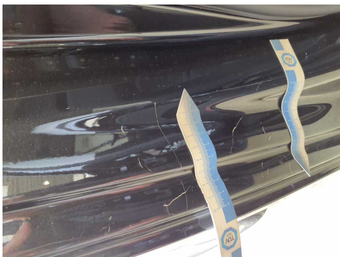
Damage 9: Side panel - rear right side: Sill - Scratch(es) - Paint
