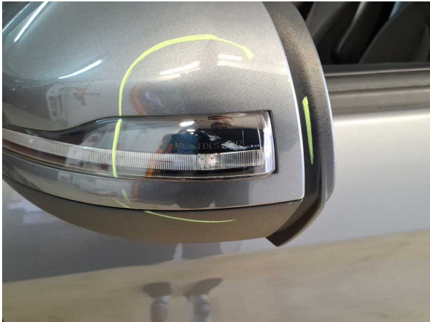
Damage #2: Indicator - front: Mirror - left side - Scratched - Replace
