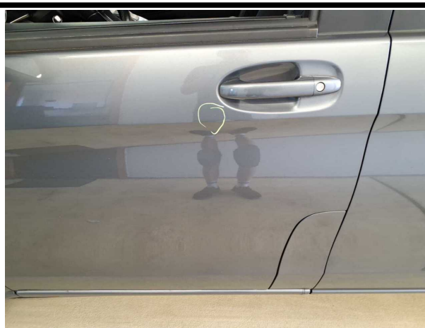
Beschädigung #6: Tür vorn links: Tür - Delle / Lackschaden - Smart Repair
