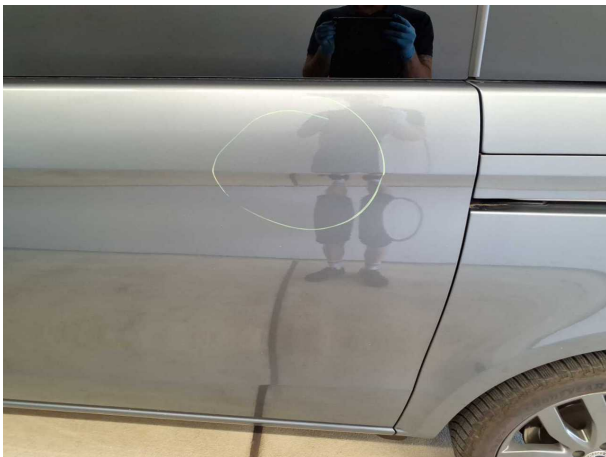
Damage #4: Sliding door - left side: Sliding door with glass panel - Dent / paintcoat damage - Smooth repair work
