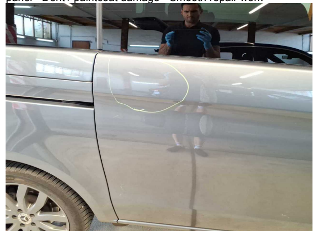
Damage #5: Sliding door, right: Sliding door with glass panel - dent(s) - Smooth repair work
