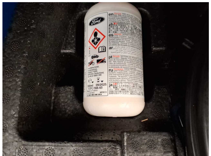
Damage 1: Equipment: Tirefit filler - Expired - Replace
