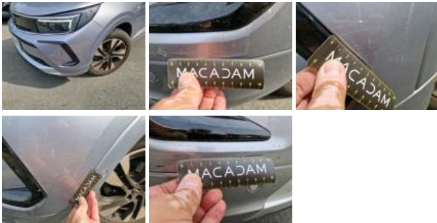
Bumper moulding FR, Scratch(es), Paint
