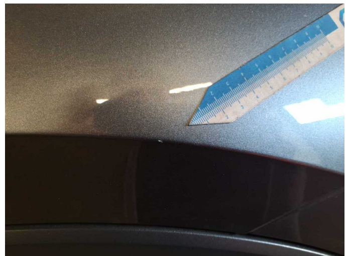
Damage 3: Mudguard - right side: Mudguard - right side - Stone chips - Smart repair
