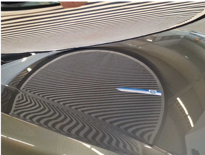
Damage 2: Bonnet: Bonnet - dent(s) - Smooth repair work
