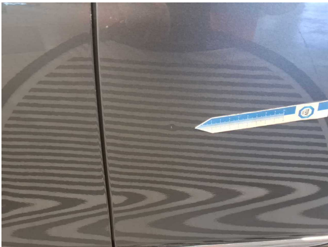
Damage 6: Door - rear left side: Door - Dent / paintcoat damage - Paint
