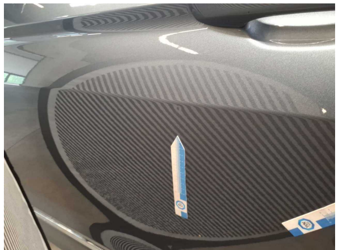
Damage 7: Door - front left side: Door - Dent / paintcoat damage - Paint
