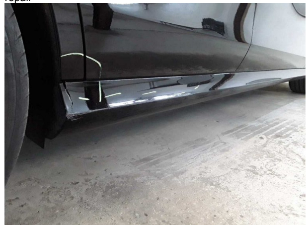
Damage #4: Sill - right side: Trim - Broken / torn - Replace
