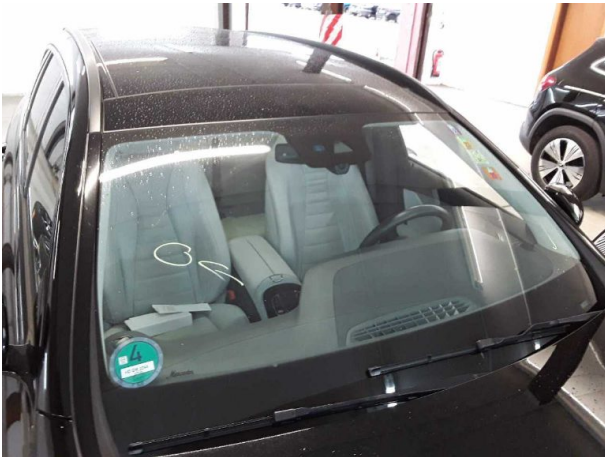
Damage #5: Vehicle glazing: Windscreen (Steinschläge) - Replace
