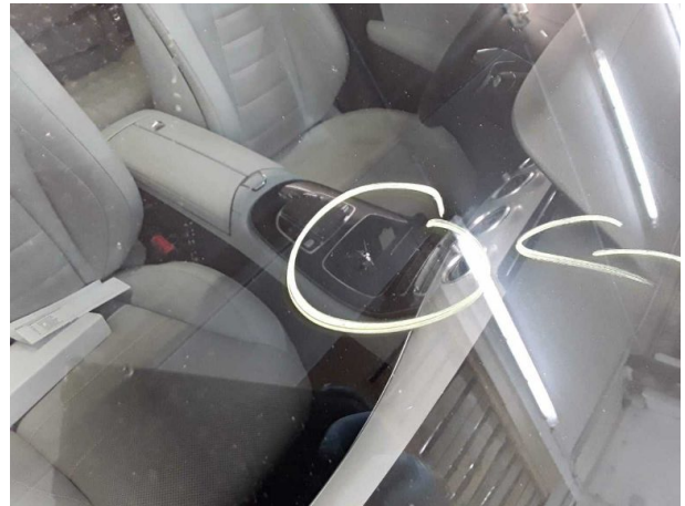
Damage #5: Vehicle glazing: Windscreen (Steinschläge) - Replace
