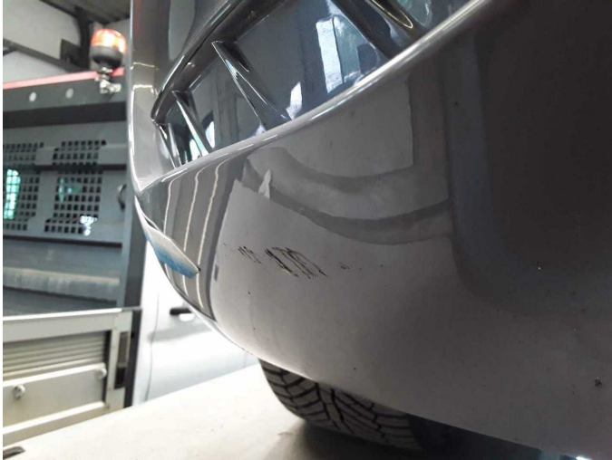
Damage 4: Rear bumper: Rear bumper - Scratch(es) - Paint
