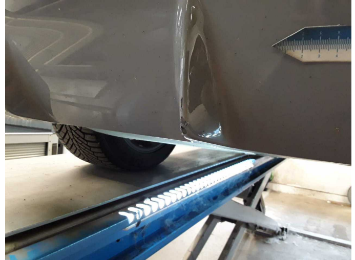
Damage 4: Rear bumper: Rear bumper - Scratch(es) - Paint
