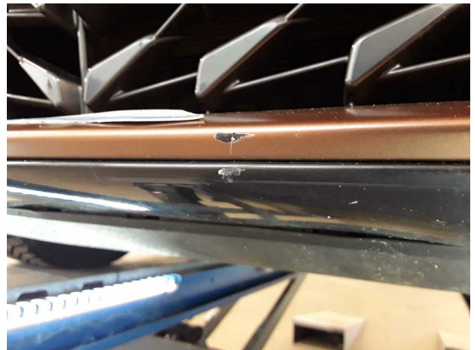
Damage 2: Front bumper: Spoiler - Scratch(es) - Smart repair
