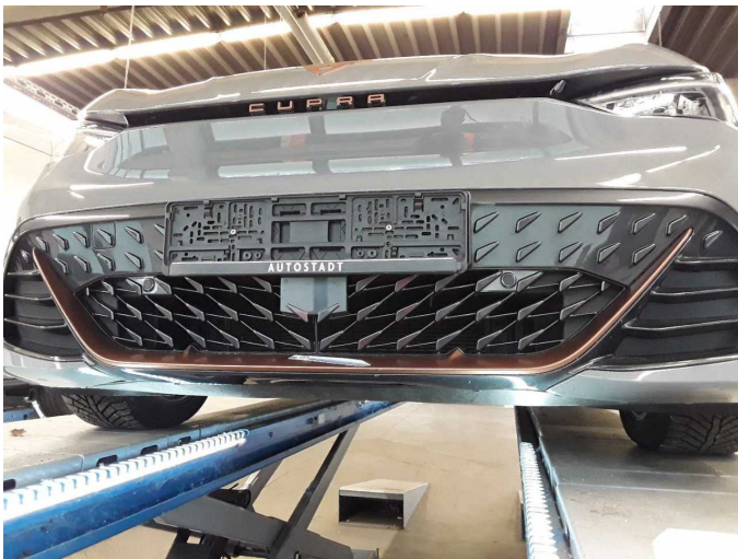
Damage 2: Front bumper: Spoiler - Scratch(es) - Smart repair
