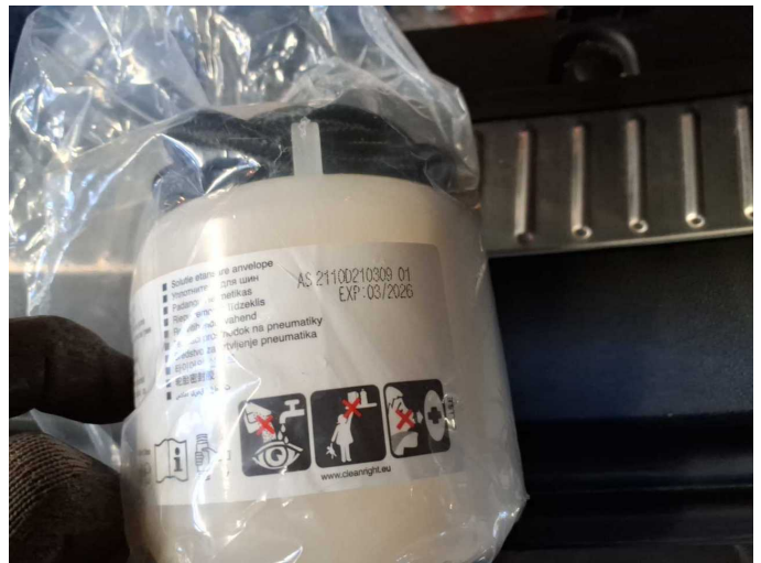
Damage 3: Equipment: Tirefit filler - Expired - Replace
