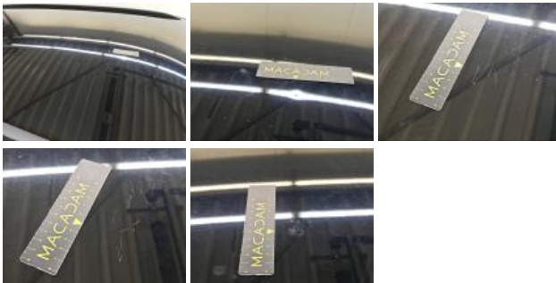
Roof, Dent(s) and scratch(es), Repair and paint (complete)
