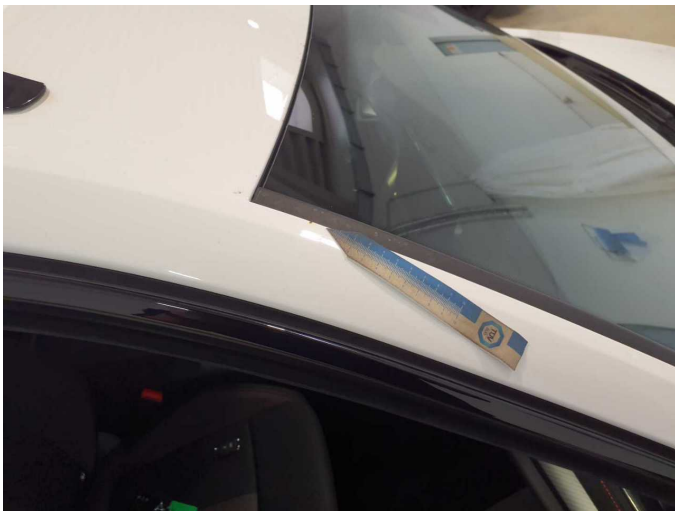
Damage 5: Body: A-pillar - right side - Corrosion - Repair and paint
