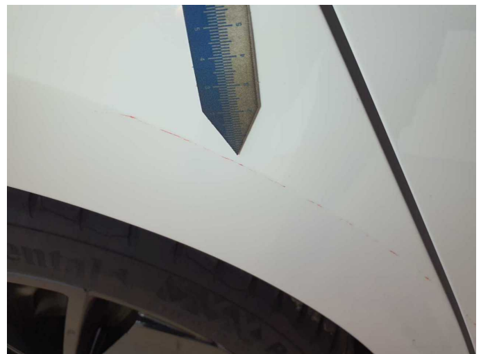
Damage 6: Side panel - rear right side: Side panel - Scratch(es) - Paint
