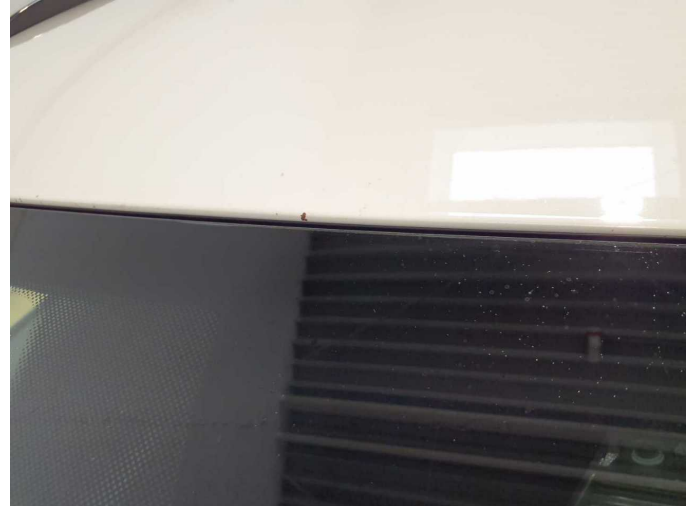
Damage 9: Roof: Roof - Corrosion - Repair and paint
