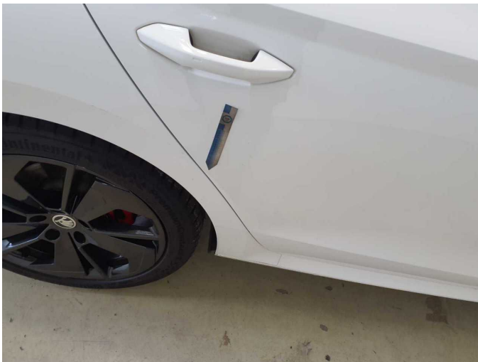
Damage 1: Door - rear right side: Door - Scratch(es) - Smart repair
