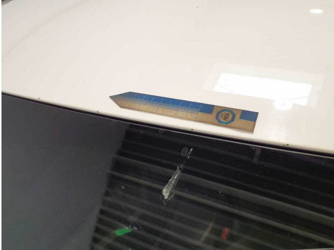
Damage 9: Roof: Roof - Corrosion - Repair and paint
