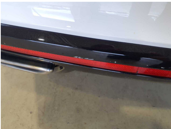
Damage 7: Rear bumper: Rear bumper (Inklusive anbauteile) - Dent / paintcoat damage - Repair and paint
