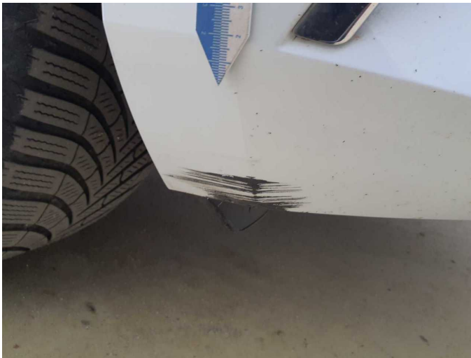
Damage 8: Front bumper: Front bumper - Scratch(es) - Paint
