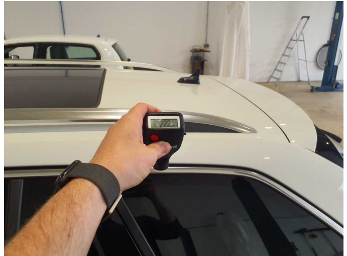
Repainting 1: Roof rail - left side
