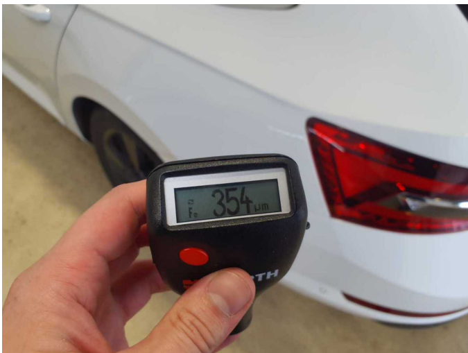
Repainting 2: Side panel - rear left side
