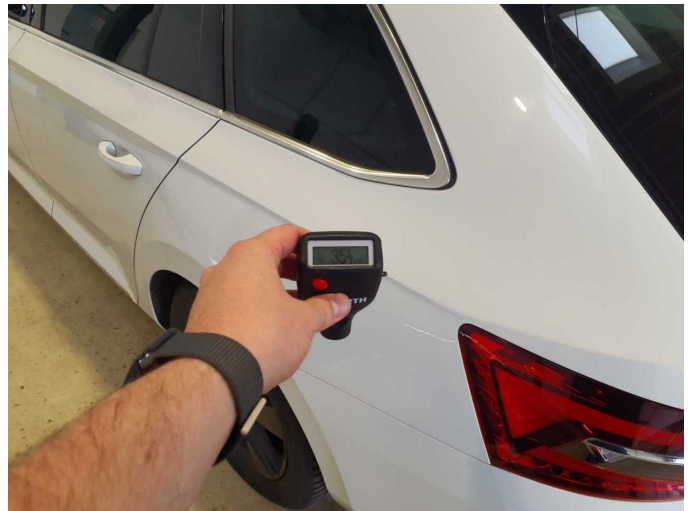
Repainting 2: Side panel - rear left side
