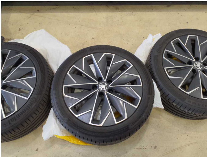
Damage 6: 2nd wheel set: 1 alloy rim - Scratch(es) - Loss in value
