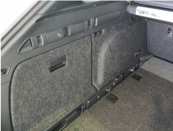
Wear and tear 4: Trim / covers: Boot lining - Abrasion - No deduction
