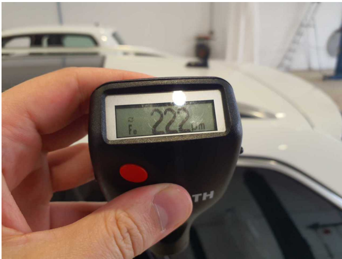
Repainting 1: Roof rail - left side
