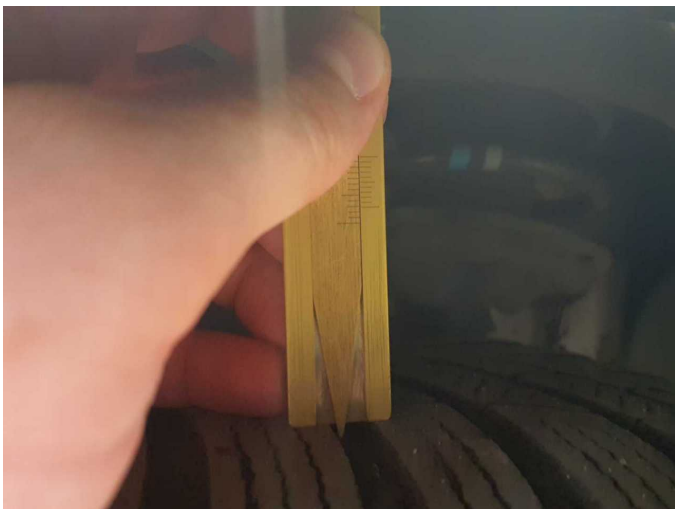
Damage 7: Wheel / tyres: Tyre - front - Worn - Replace
