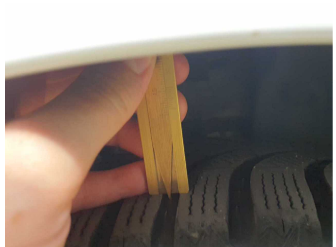
Damage 7: Wheel / tyres: Tyre - front - Worn - Replace
