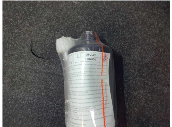
Damage 2: Equipment: Tirefit filler - Expired - Replace
