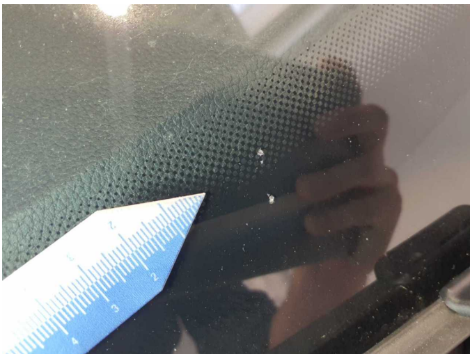
Damage 11: Vehicle glazing: Windscreen - Stone chips - Replace
