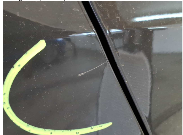
Damage #9: Side panel - rear right side: Side panel - Scratch(es) - Repair and paint
