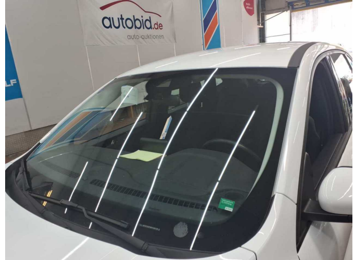
Damage 3: Vehicle glazing: Windscreen - Stone chips - Replace
