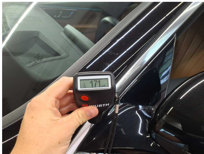
Repainting 1: Roof rail - left side
