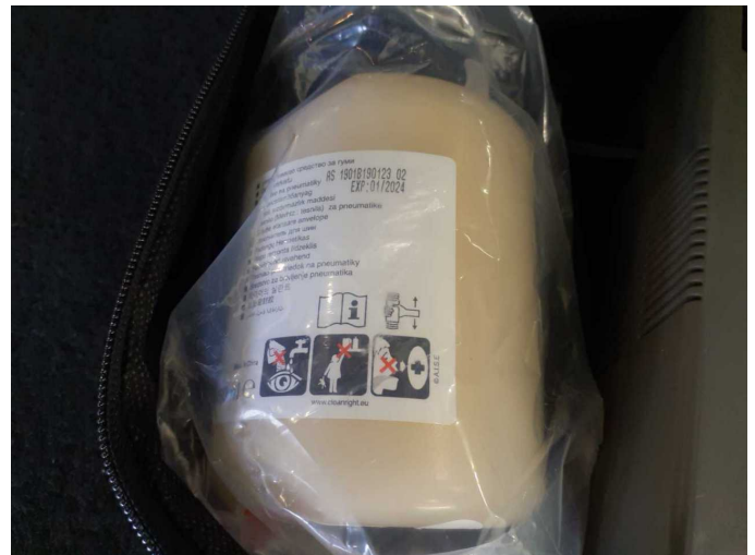
Damage 1: Equipment: Tirefit filler - Expired - Replace
