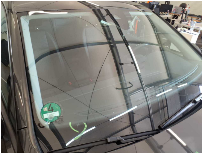
Damage 8: Vehicle glazing: Windscreen - Stone chips - Replace
