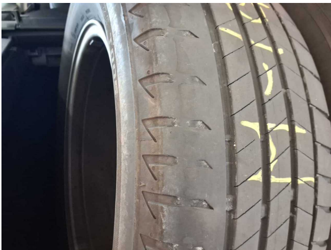
Damage 2: 2nd wheel set: 1 tyre - Worn - Replace
