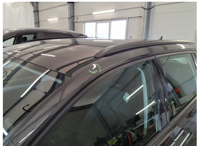
Damage 7: Body: Body - Damage by hail - Smart repair
