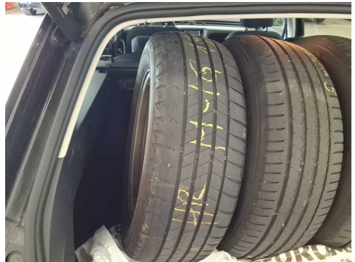
Damage 2: 2nd wheel set: 1 tyre - Worn - Replace
