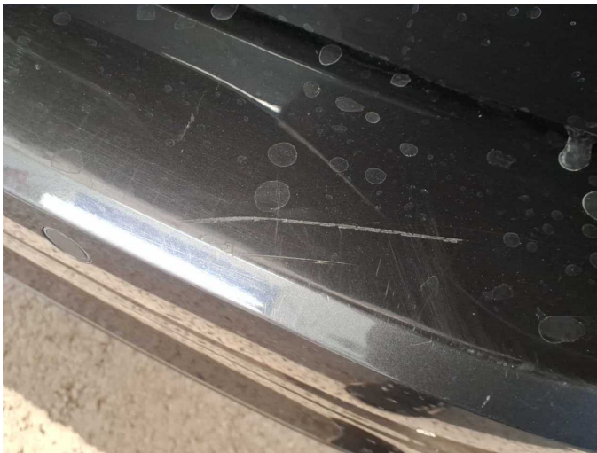
Damage 5: Rear bumper: Rear bumper - Scratch(es) - Paint
