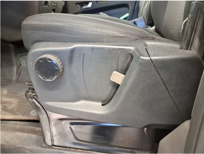
Damage 1: Seat - front: Lever seat adjustment - Missing - Replace
