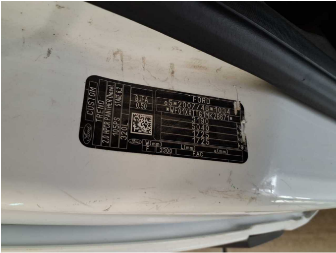
Damage 2: Body: Identification plate - Scratch(es) - Replace
