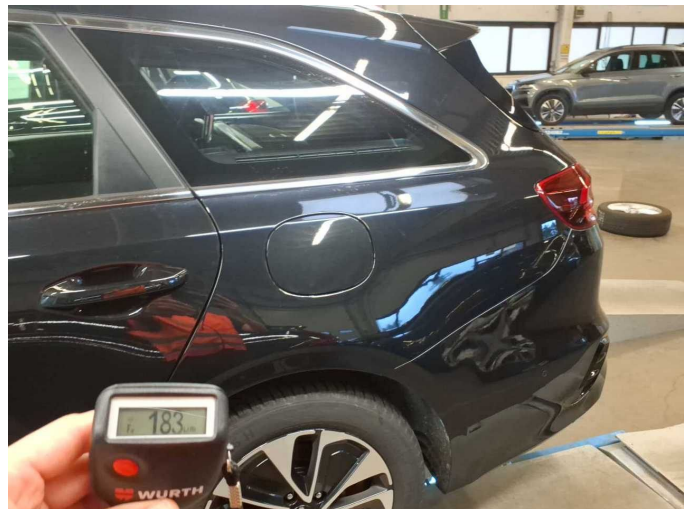
Repainting 1: Side panel - rear left side
