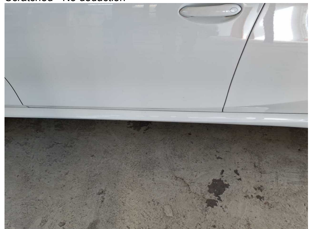
Damage #4: Sill - left side: Trim - Scratched - Repair and paint
