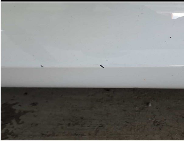
Damage #4: Sill - left side: Trim - Scratched - Repair and paint
