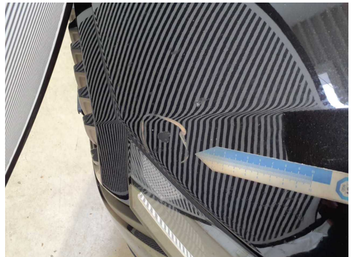
Damage 7: Bonnet: Bonnet (Lack löst sich) - Unprofessionally repaired - Repair and paint
