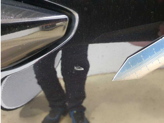
Damage 6: Door - front right side: Door - Dent / paintcoat damage - Repair and paint
