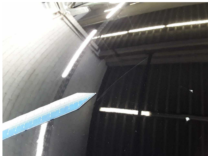
Damage 6: Bonnet: Bonnet - Scratch(es) - Paint
